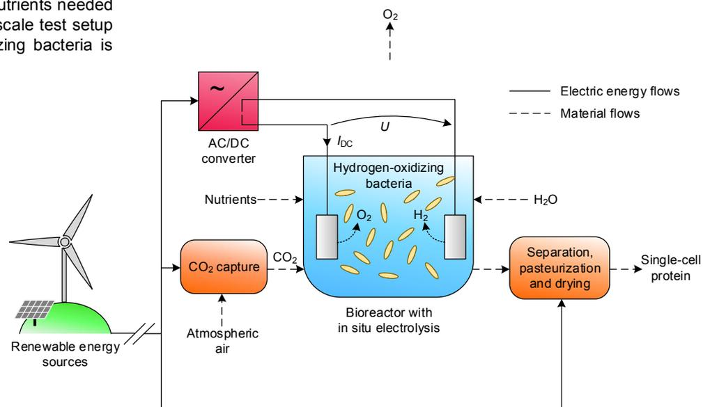
Figure 2. Scheme of the concept of producing microbial protein from electricity, water, air, and nutrients
