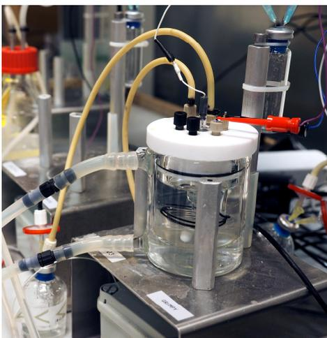
Figure 1. Laboratory scale test setup for in-situ electrolysis cultivation of hydrogen oxidizing bacteria.
